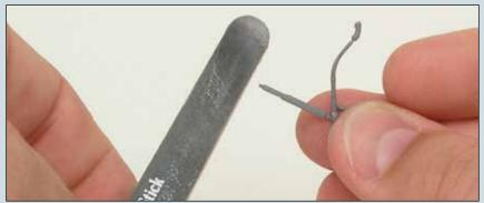
2. Sand away mold lines (left over from the injection-molding process) and any other irregularities on the part before gluing it.
